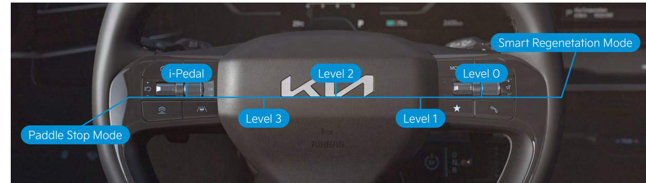
Pedal Stop Mode, i-Pedal, Level 3, Level 2, Level 1, Level 0, and Smart Regeneration Mode. These are the names of our seven regenerative braking levels that can be activated via steering-wheel paddles.
